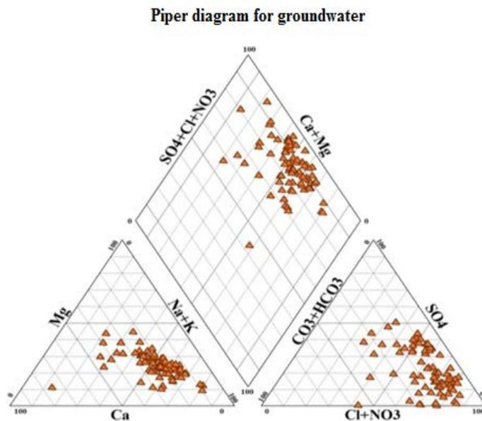
Figure 2: Piper diagram for irrigation water of Oued El Maleh.
