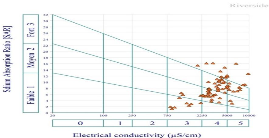
Figure 3: Diagram for determination of the quality of irrigation water
